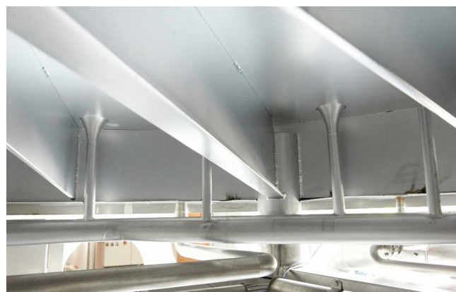
Figure 4: With the current false bottom distance and the flow-optimized tulip pipes, the collection area can be increased to 2.5 m 2 – without compromising the yield or wort quality.
