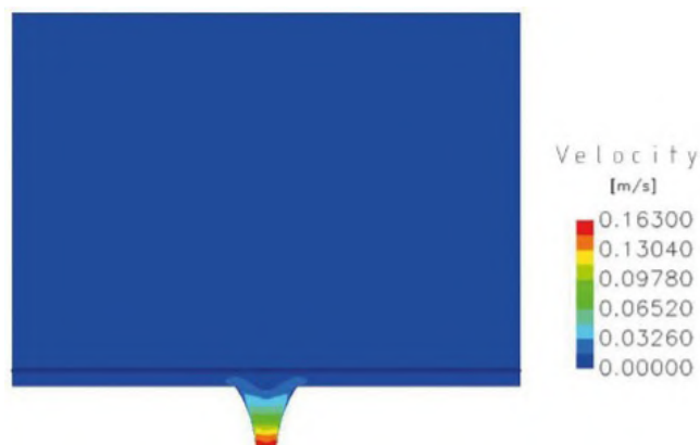
Figure 3: With an optimal design of the "tulip" pipes and the current false bottom distance, the spent grains cake is no longer affected by a partial suction effect.
