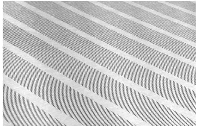
Figure 1: This second, perforated false bottom is installed above the actual bottom of the lauter tun
