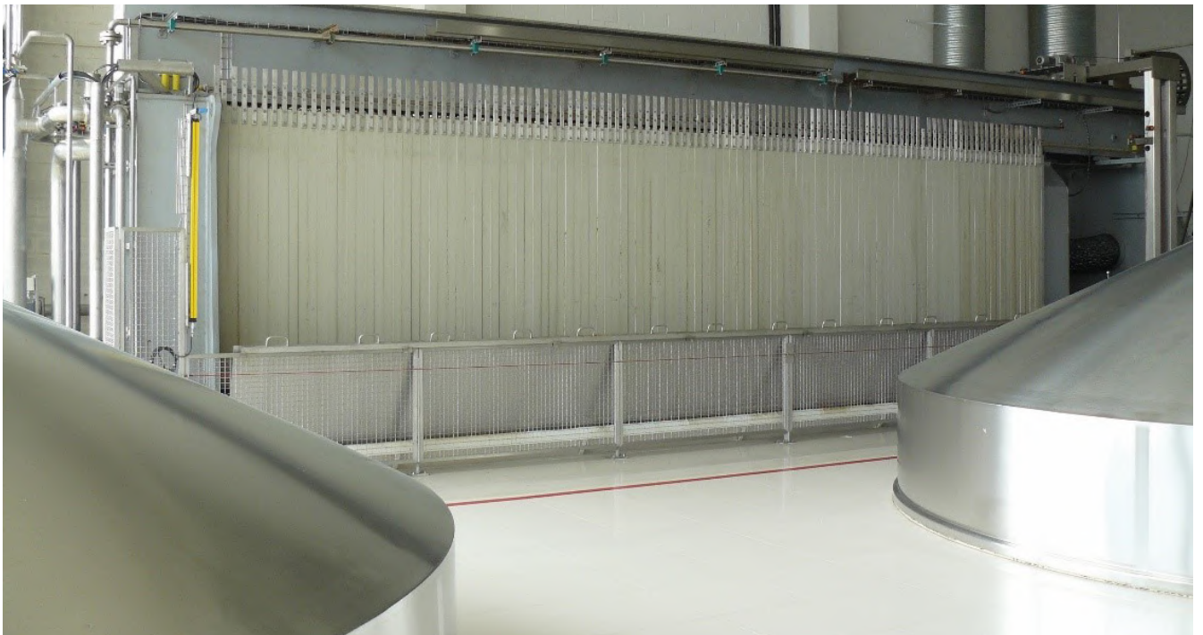
Figure 5: In the mash filter the entire spent grains is divided into many vertical spent grains' cakes.
