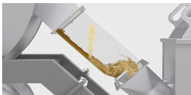
Figure13b: An integrated baffle plate creates turbulences, resulting in an improved mixing of the spent grains and thus leading to an effective extraction.
