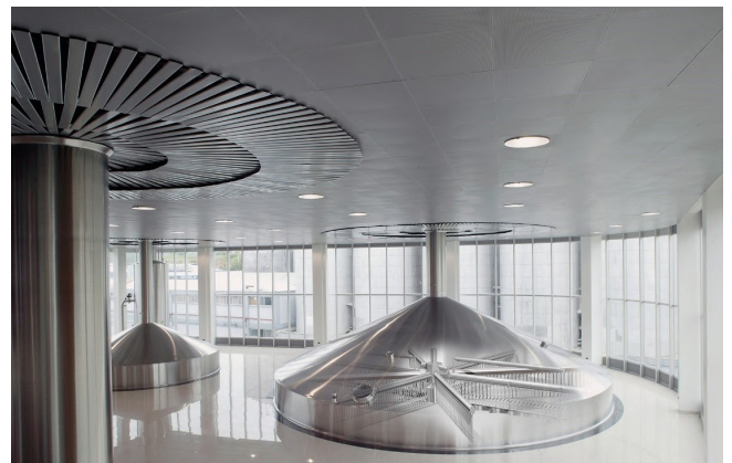
Figure 2: Today's lauter tuns can achieve peak values of up to 14 brews per day.
