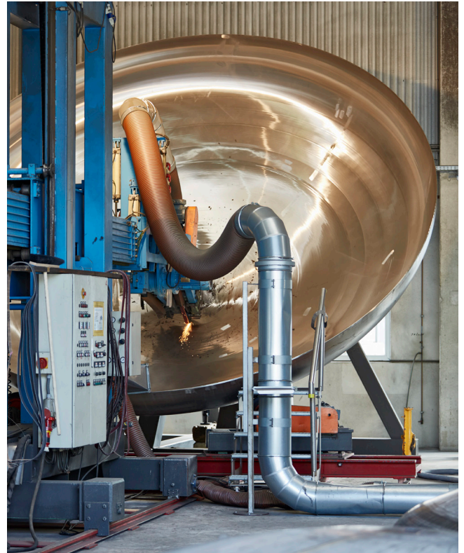
Figure 5: Surfaces of tanks are polished to a surface roughness of less than 0.8 \mu\text{m}
